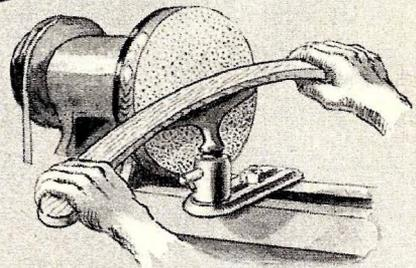
SANDPAPER GLUED TO WOODEN DISK AND FASTENED TO FACE PLATE
