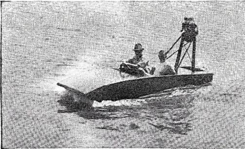
Driven by an airplane propeller fitted to a motorcycle engine mounted at rear, H. V. Kenna's "Whizzer" travels 20 m.p.h.
