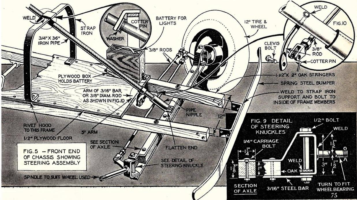
FIG. 5 - FRONT END OF CHASSIS SHOWING STEERING ASSEMBLY
