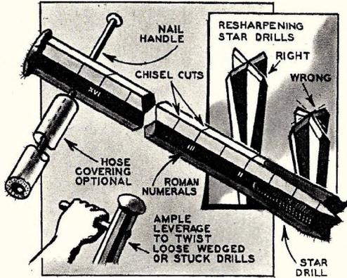
IF THE shank of a star drill is marked off in inch and half-inch notches, it will always indicate its depth in the hole it is making, eliminating the necessity for measuring drilling progress with a ruler. Either Roman numerals or just scratches can be used to indicate depth. When taking readings, allow for shortening of the drill by sharpening.
