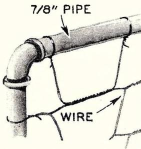
This sweet-pea trellis of galvanized pipe and wire can be pulled up and moved to a new spot each season. When the vines have withered the trellis can be pulled up and stored to make room for any other plants.
