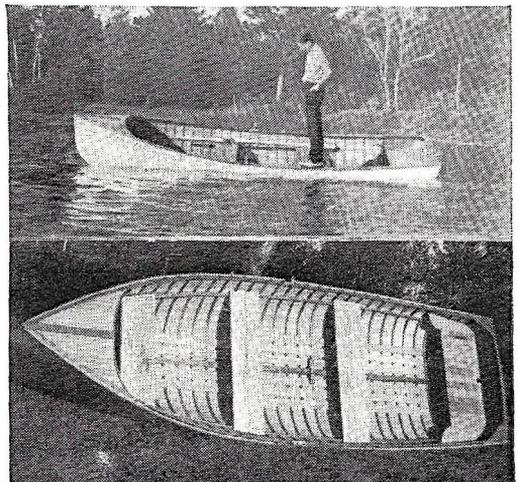
James W. Spoor's home-built 15-foot round bottom boat is so stable that a man can stand on the gunwale (top) without capsizing it. Lower photo shows construction details.
