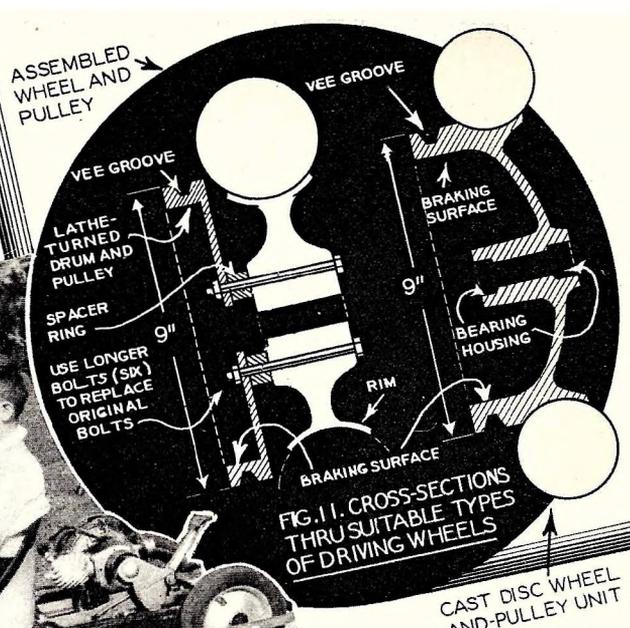
FIG. 11. CROSS-SECTIONS THRU SUITABLE TYPES OF DRIVING WHEELS
