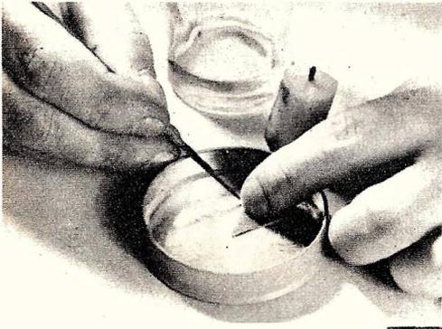
The triangular opening can be made by scratching dimensions in wax over the bottom and filling it with acid. After a few minutes, it will fall out.
