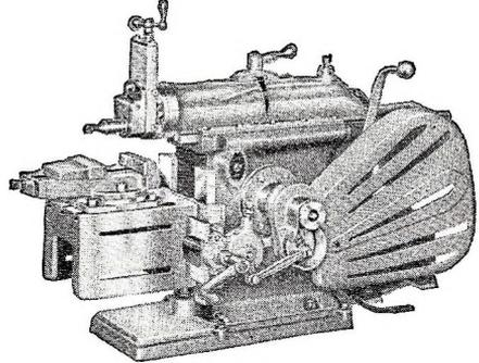
A seven-inch shaper incorporating principles of modern shaper construction. Four speeds, between forty-five and 200 strokes a minute are available.
