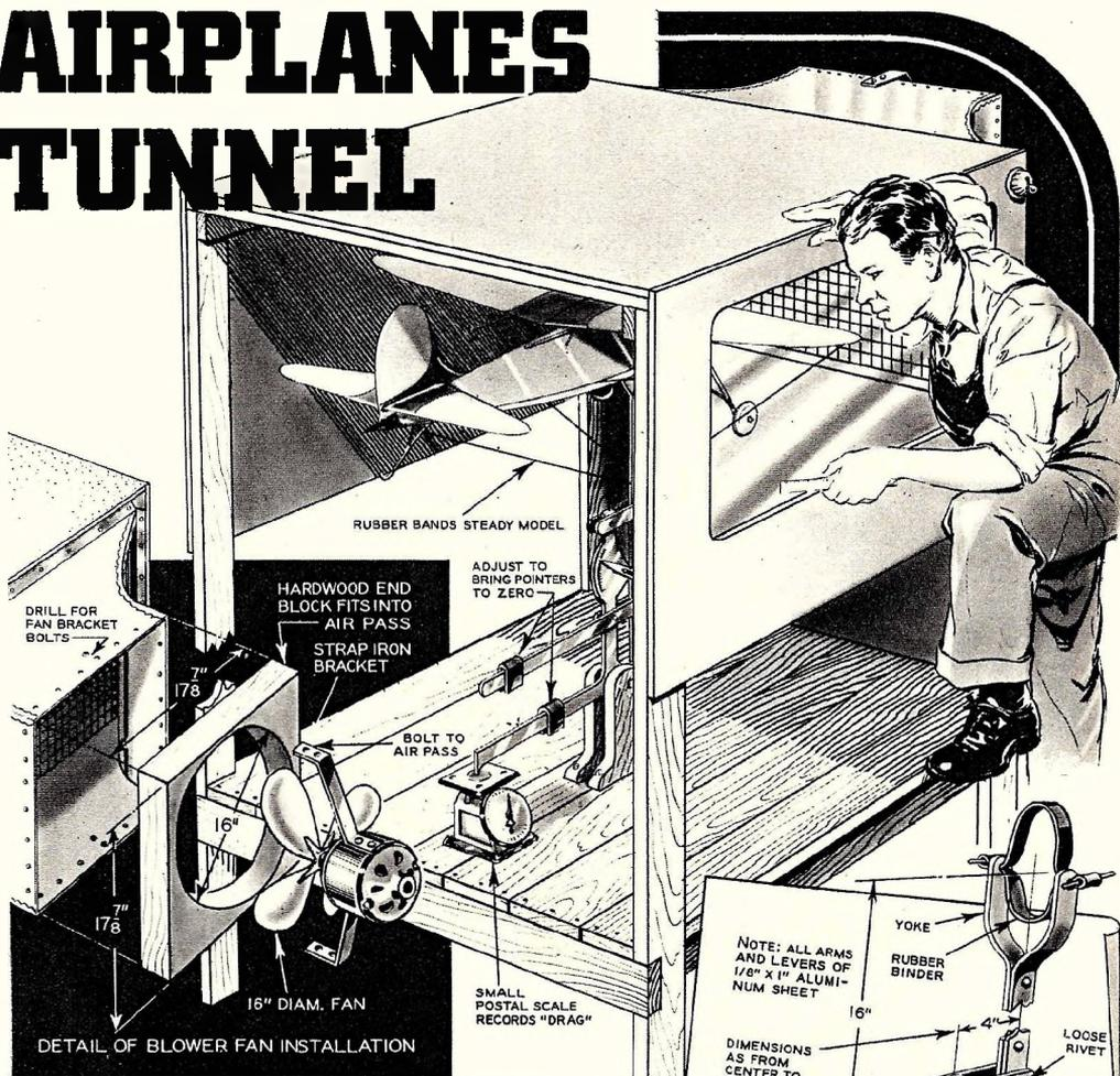
trating the complete wind tunnel assembly.
