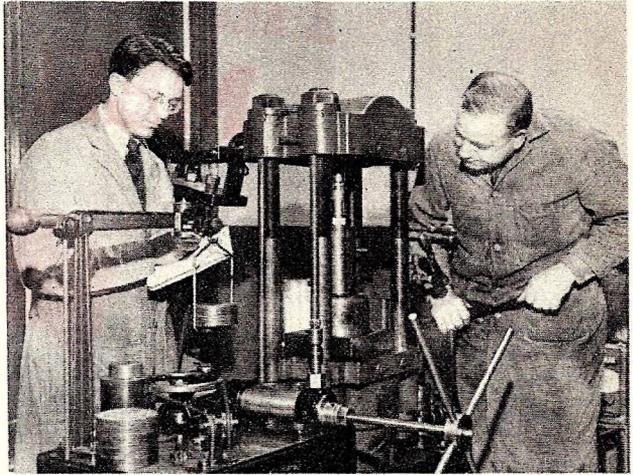
With this tool, pressures up to 1,500,000 pounds per square inch are possible. This new device opens new fields of research including the behavior of untapped energy in the atom and the earth's structure 200 miles down.
