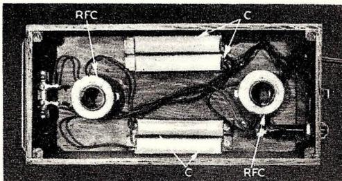
An under view of the filter baseboard showing the parts. The fuse is in the tube at the lower right side. The two choke coils are mounted in the center, and condensers at sides. Note the wiring simplicity.
