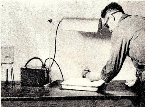
The adjustable mounting of this new ultra-violet ray lamp enables the operator to direct the radiations where desired.
