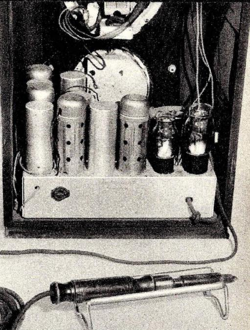
The fused line filter in use takes up very little room and gives protection against blowing house fuses.
