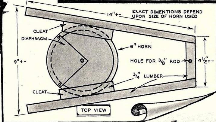
**T**HIS small and easily constructed jig saw, built from some scrap wood, a discarded auto horn, and part of an old carburetor, has been found to cut balsa wood accurately and quickly and has proved entirely satisfactory for the model airplane worker. By using very fine scroll blades, this saw will run on six to eight volts from a toy transformer for a considerable time without overheating and will cut one-half-inch balsa cleanly and quickly.
