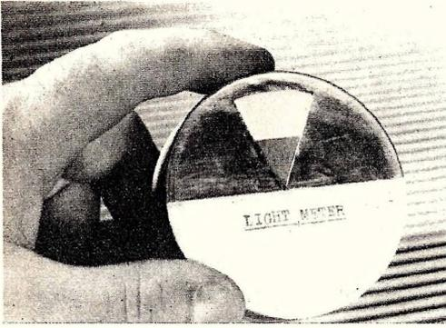
A round typewriter ribbon box makes a satisfactory holder for the light meter. With this device it is easy to test the light-giving qualities of a reading lamp. Of simple construction, it is even easier to use and gives satisfactory results.
