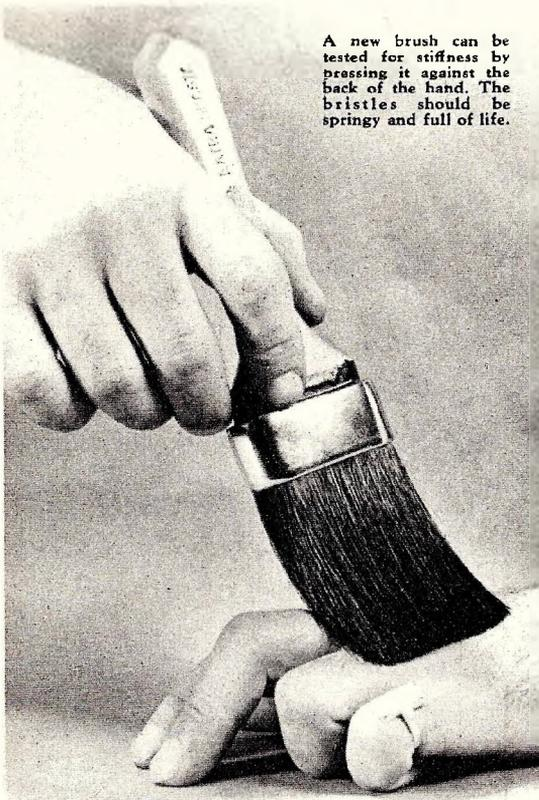
A new brush can be tested for stiffness by pressing it against the back of the hand. The bristles should be springy and full of life.
