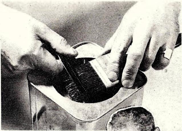
Above—Use a coarse comb to work the cleaner deep into the heel so that every trace of paint is removed. Above right—The result of improper cleaning and care of what was a good brush.
