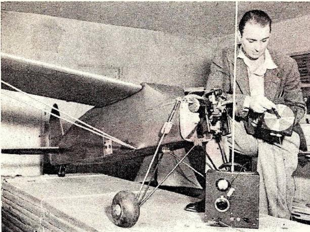
Paul Whittier, veteran pilot, examines the ground radio equipment which will be used to control this 12-foot gasoline-powered model when it is used as a flying target during coast artillery maneuvers to be held in California.
