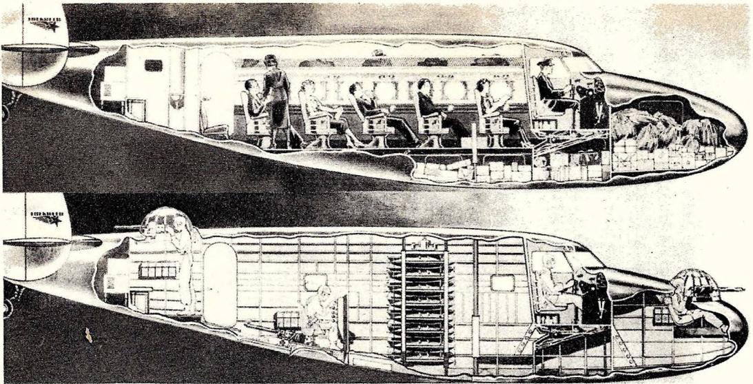
Many modern commercial airplanes are so designed that they can easily and quickly be converted into bombing planes in event of war. The cross-section sketches above show conversion of Lockheed transport.
