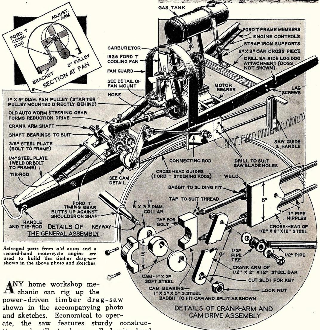
Salvaged parts from old autos and a second-hand motorcycle engine are used to build the timber drag-saw shown in the above photo and sketches.
