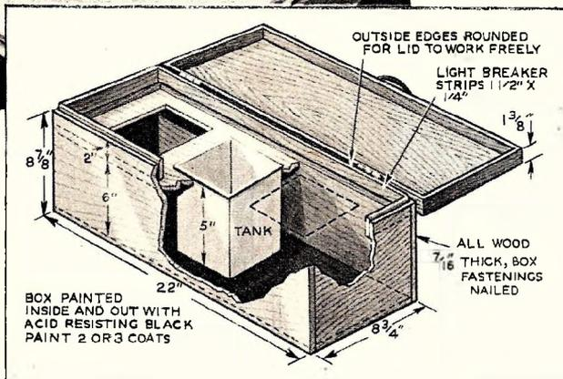
when the lid is down. Thus, after placing of the film in the developer, and the lid closed, the darkroom lights may be turned on and other work done while the negatives develop and fix. Regular Kodak film developing hangers are used, which, when used with the No. 1 developing box, will handle any cut film size up to 4x5 inches.
