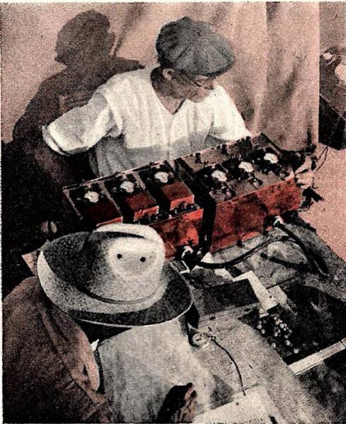
Here is a battery of electrically controlled stop watches. Large charts are kept and every lap accurately recorded. Every possible precaution is taken to prevent slightest error in records.
