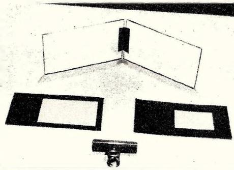
Masks for use with the hinged optical glass negative holder are cut from black paper, as shown above. The spring-type paper clip serves as a handle for the holder.
