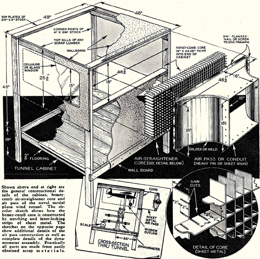
Shown above and at right are the general constructional details of the cabinet, honeycomb air-straightener core and air pass of the novel model plane wind tunnel. The circular sketch shows how the honeycomb core is constructed by notching and inter-locking strips of sheet metal. The sketches on the opposite page show additional details of the air pass construction as well as complete details of the dynamometer assembly. Practically all parts are made from easily obtained scrap materials.
