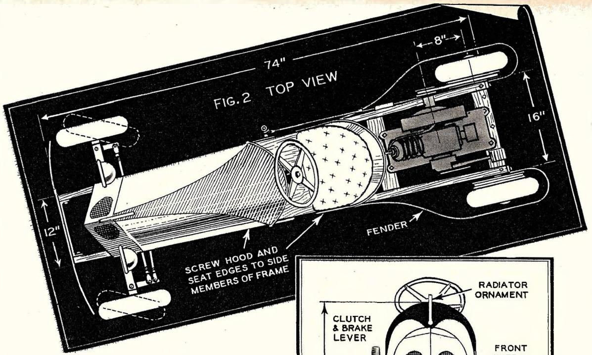
the edges of the metal should be beaded. The edge of the seat back is protected with a strip of leather laced on with rawhide. It will be best to leave the cutting of the hood, etc., until the chassis is completed.
