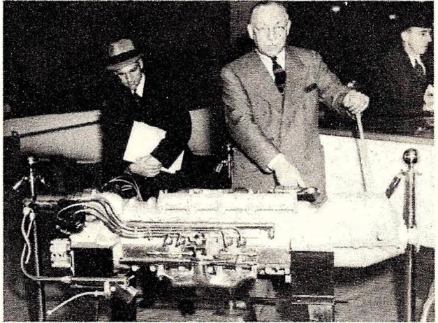
Developing 125 horsepower, this new marine gasoline turbine features firing and compression rotors instead of pistons and fires four times as much as an ordinary gasoline engine.
