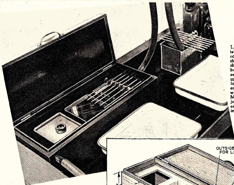
Left—Set-up of the finished box in the darkroom. Water runs in through one pipe at the right end of the box, and out through another pipe in the upper left corner. Below—This developing outfit is a very simple wood-working project. Minor leakage at the joints is not important, as the box is kept in a sink anyway.
