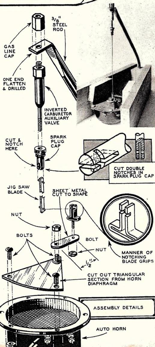
Easy to construct, this jig saw will be found very helpful to the model airplane builder. It will cut balsa up to one-half an inch thick. Six to eight volts from a stepdown transformer will power it.
