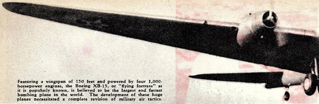
Featuring a wingspan of 150 feet and powered by four 1,000-horsepower engines, the Boeing XB-15, or "flying fortress" as it is popularly known, is believed to be the largest and fastest bombing plane in the world. The development of these huge planes necessitated a complete revision of military air tactics.
