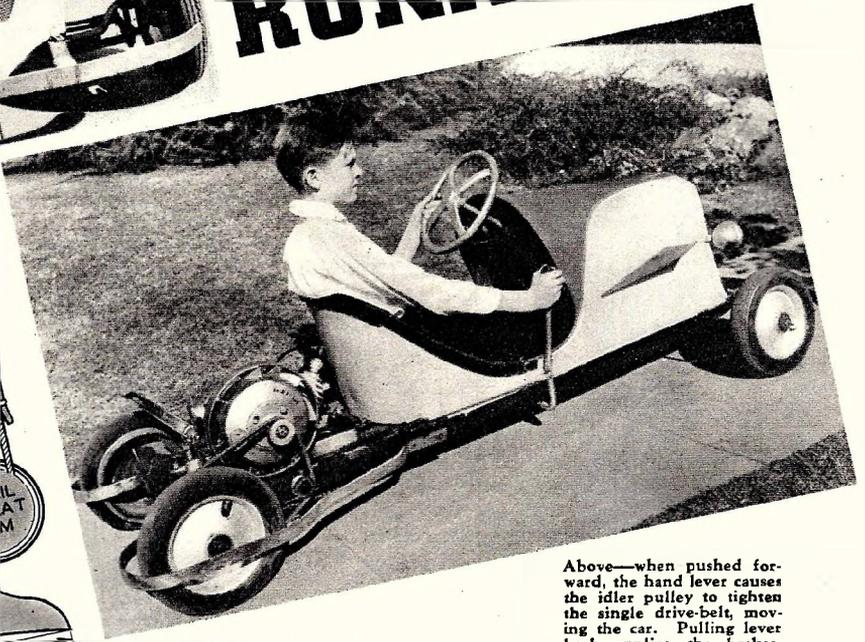
Above—when pushed forward, the hand lever causes the idler pulley to tighten the single drive-belt, moving the car. Pulling lever back applies the brakes.
