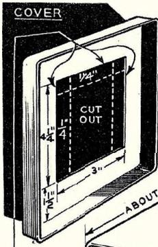
The cover of the tin can lamp housing is cut out, as shown in sketch at left, after which the housing is soldered to the negative holder box, making a firm, light-tight assembly. Construction details of the easel and baseboard assembly are shown in the sketch at lower right.
