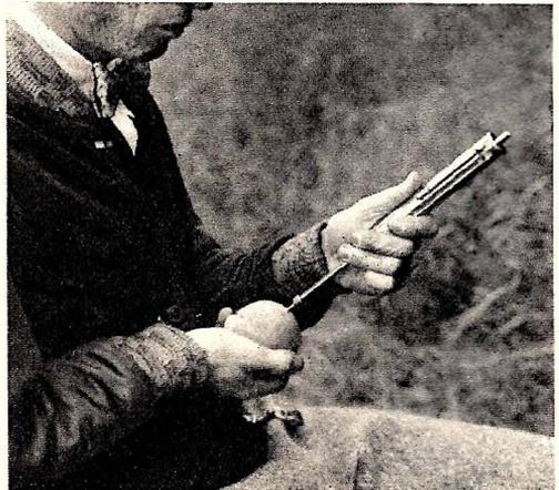
Pushed into a peach, this scientific tester has a calibrated scale that accurately indicates the ripeness of the fruit.
