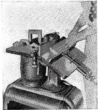
Featuring a tilting table which is raised or lowered on an accurately ground column, a new shaping machine makes it possible to cut bevels and intricate moulding with standard shaper knives. Manufactured by a Wisconsin firm, the shaper can be had as a bench or floor type.
