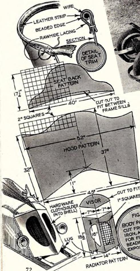
**T**HERE is one definite rule to follow in making a sidewalk automobile—get your engine first and build the car around it. This applies pretty much to the wheels, too.
